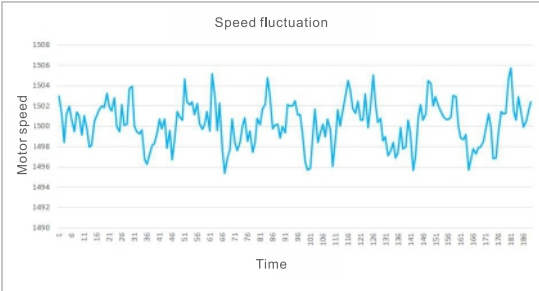
The speed fluctuation of VH6 series frequency converter driving the motor at rated torque and speed is stable at ±0.2%.
